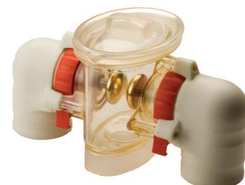
400 ml vessel assembly (electrodes fitted)
